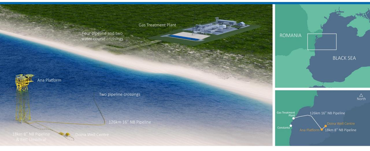
• 10 Bcm Resources • 1 Platform with 4 wells • 1 Subsea well • 126km transport pipeline • Onshore gas plant
